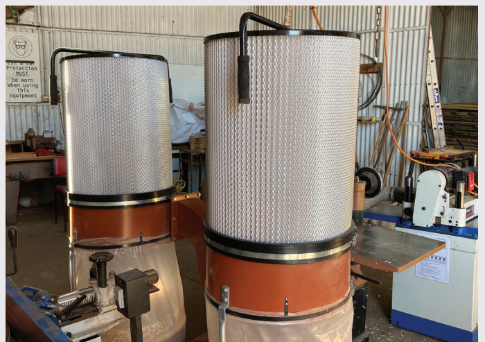
New dust filters have dramatically improved conditions at the Benalla Woodworkers’ Association.
